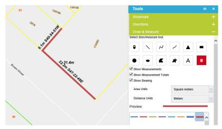
Fig.56 Draw & Measure Tool – Polyline drawing showing segment lengths, bearing and total length
