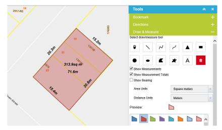
Fig.58 Draw & Measure Tool – Polygon drawing showing sides' lengths, total length and Area
